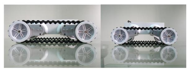
Each gearbox has an 87:1 ratio includes an optical quadrature encoder that gives 1000 pulses over 3 revolutions of the output shaft. The chassis can be upgraded to include four motors and encoders making it ideal for mecanum wheels.
