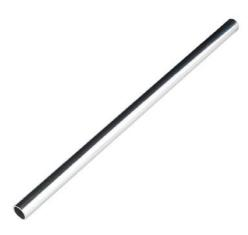
**Description:** These 8" long aluminum tubes have an outer diameter of 3/8", an inner diameter of 0.30", and a wall thickness of 0.035". When used with the mating tube clamps, these can be used for versatile structural support. Additionally, wires and cables can easily be run through the center.
