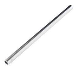
**Description:** These 18" long aluminum tubes have an outer diameter of 1", an inner diameter of 0.82", and a wall thickness of 0.09". When used with the mating tube clamps, these can be used for versatile structural support. Additionally, wires and cables can easily be run through the center.
