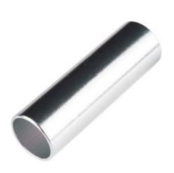
**Description:** These 2" long aluminum tubes have an outer diameter of 5/8", an inner diameter of 0.569", and a wall thickness of 0.028". When used with the mating tube clamps, these can be used for versatile structural support. Additionally, wires and cables can easily be run through the center.
