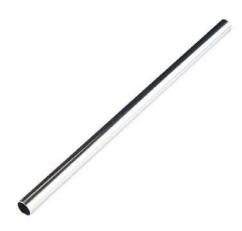
**Description:** These 10" long aluminum tubes have an outer diameter of  $\frac{1}{2}$ ", an inner diameter of 0.444", and a wall thickness of 0.03". When used with the mating tube clamps, these can be used for versatile structural support. Additionally, wires and cables can easily be run through the center.
