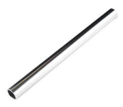
**Description:** These 12" long aluminum tubes have an outer diameter of 1", an inner diameter of 0.82", and a wall thickness of 0.09". When used with the mating tube clamps, these can be used for versatile structural support. Additionally, wires and cables can easily be run through the center.
