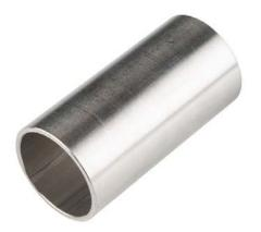
**Description:** These 2" long stainless steel tubes have an outer diameter of 1", an inner diameter of 0.88", and a wall thickness of 0.06". When used with the mating tube clamps, these can be used for versatile structural support. Additionally, wires and cables can easily be run through the center.
