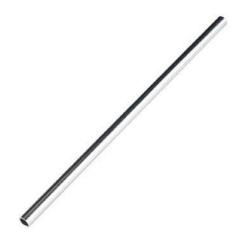
**Description:** These 10" long aluminum tubes have an outer diameter of 3/8", an inner diameter of 0.30", and a wall thickness of 0.035". When used with the mating tube clamps, these can be used for versatile structural support. Additionally, wires and cables can easily be run through the center.
