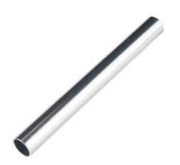
**Description:** These 6" long aluminum tubes have an outer diameter of 5/8", an inner diameter of 0.569", and a wall thickness of 0.028". When used with the mating tube clamps, these can be used for versatile structural support. Additionally, wires and cables can easily be run through the center.
