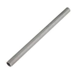
**Description:** These 10" long aluminum tubes have an outer diameter of 5/8", an inner diameter of 0.569", and a wall thickness of 0.028". When used with the mating tube clamps, these can be used for versatile structural support. Additionally, wires and cables can easily be run through the center.
