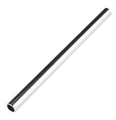
**Description:** These 6" long aluminum tubes have an outer diameter of 3/8", an inner diameter of 0.30", and a wall thickness of 0.035". When used with the mating tube clamps, these can be used for versatile structural support. Additionally, wires and cables can easily be run through the center.
