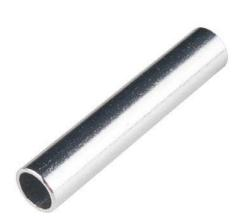
**Description:** These 2" long aluminum tubes have an outer diameter of 3/8", an inner diameter of 0.30", and a wall thickness of 0.035". When used with the mating tube clamps, these can be used for versatile structural support. Additionally, wires and cables can easily be run through the center.
