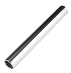
**Description:** These 8" long aluminum tubes have an outer diameter of 1", an inner diameter of 0.82", and a wall thickness of 0.09". When used with the mating tube clamps, these can be used for versatile structural support. Additionally, wires and cables can easily be run through the center.
