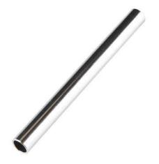
**Description:** These 4" long aluminum tubes have an outer diameter of 3/8", an inner diameter of 0.30", and a wall thickness of 0.035". When used with the mating tube clamps, these can be used for versatile structural support. Additionally, wires and cables can easily be run through the center.
