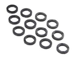
**Description:** These plastic shaft spacers have an inner diameter of 1/4" and a thickness of 1/16". These spacers are ideal for spacing out an area between a bearing and a shaft collar to reduce metal to metal contact.
