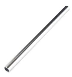
**Description:** These 16" long aluminum tubes have an outer diameter of 1", an inner diameter of 0.82", and a wall thickness of 0.09". When used with the mating tube clamps, these can be used for versatile structural support. Additionally, wires and cables can easily be run through the center.
