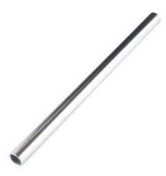
**Description:** These 14" long aluminum tubes have an outer diameter of 1", an inner diameter of 0.82", and a wall thickness of 0.09". When used with the mating tube clamps, these can be used for versatile structural support. Additionally, wires and cables can easily be run through the center.
