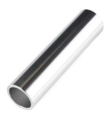
**Description:** These 4" long aluminum tubes have an outer diameter of 1", an inner diameter of 0.82", and a wall thickness of 0.09". When used with the mating tube clamps, these can be used for versatile structural support. Additionally, wires and cables can easily be run through the center.
