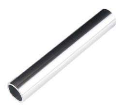
**Description:** These 6" long aluminum tubes have an outer diameter of 1", an inner diameter of 0.82", and a wall thickness of 0.09". When used with the mating tube clamps, these can be used for versatile structural support. Additionally, wires and cables can easily be run through the center.
