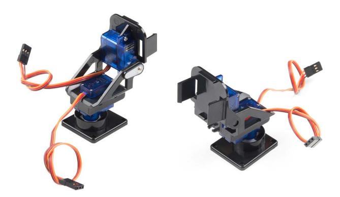
This is an easy-to-assemble pan/tilt bracket kit that utilizes servos to move on two axes fit for camera and helping-hand applications. This particular bracket kit is the same one we use in our SparkFun Raspberry Pi Zero W Camera Kit to create a remote camera system for your home or workplace.
