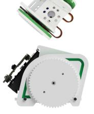
**STEP 3:** Push the SERVO:LITE board fully back inside the :MOVE mini.
