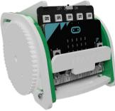
**STEP 4:** Secure the SERVO:LITE board and micro:bit with the :MOVE T-piece.
