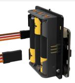
**STEP 1:** Plug the servo cables back into the SERVO:LITE board. The left servo should plug into the left-hand side of the :MOVE board and vice versa. The cables should be threaded down the gaps on either side as shown and any excess tucked under the pen mounting plate.
