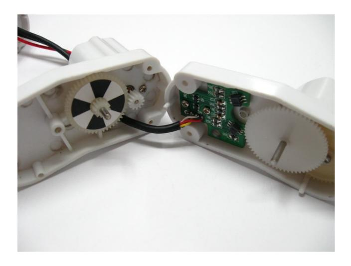
Each motor housing has two thick power wires that go directly to the motor. There are also 4 small wires with female headers.
