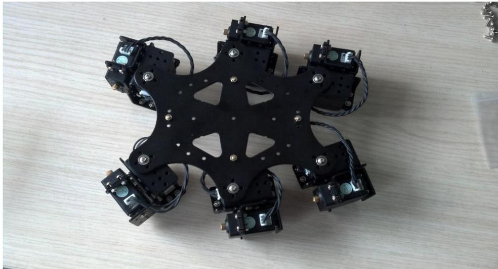
Turn over and put the back on, make sure that the servos and the servo horns are correct with each other.
