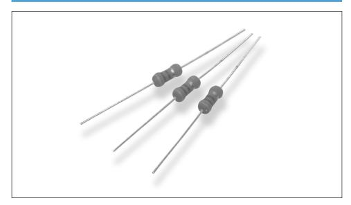
The resistive element comprises a metal oxide film deposited on a ceramic former. The element is protected by a flameproof coating which will withstand overload conditions without flame or mechanical damage. They are recommended for use in applications such as line protection etc...
