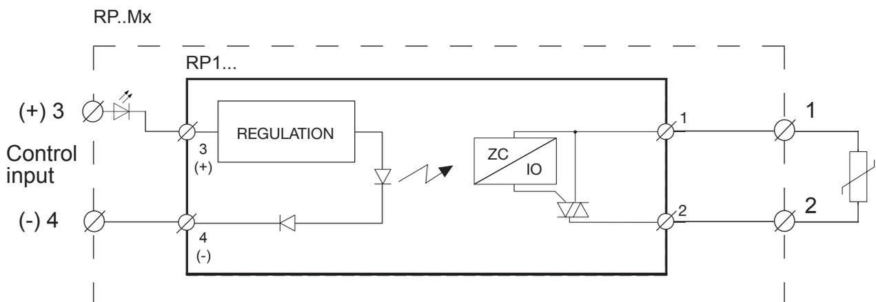
\* The varistor is not included in the solid state relay. Connecting a varistor across terminals 1-2 helps protect the solid state relay against damages by over-voltage
