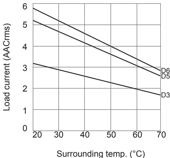
Derating curve is used for finding max. load current at an elevated ambient temperature. The 3 lines in the graph represent the 3 nominal current ratings of the RP1 series (RP1...D3/D5/D6). When used at full load current, the relays must be placed vertically. If more than one relay is mounted, please allow a minimum distance of 20 mm in between for sufficient air cooling.
