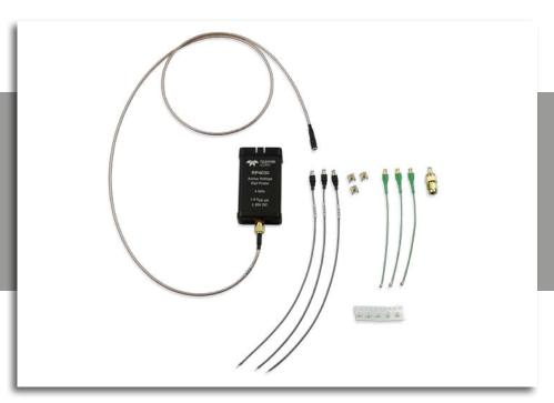
The RP4030 is designed specifically to probe a  $50\Omega$  DC power/voltage rail. The probe has large built-in offset, low attenuation (noise), and high DC input impedance. Built-in offset and low attenuation permit the power/voltage rail to be offset in the oscilloscope by its mean DC voltage with high oscilloscope gain (sensitivity) to achieve a noise-free view of small signal variations. The high DC input impedance eliminates loading of the DC rail.
