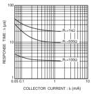
Fig.8 Response time vs. collector current
