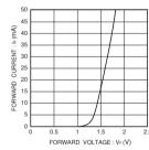
Fig.3 Forward current vs. forward voltage
