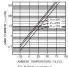
Fig.9 Dark current vs. ambient temperature
