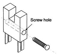
As for the above type, there is the possibility that makes electrically short-circuit between parts to Metal mounting plate, when tighten at the time of attachment and torque be strong. Especially attention to the following point and please use.
