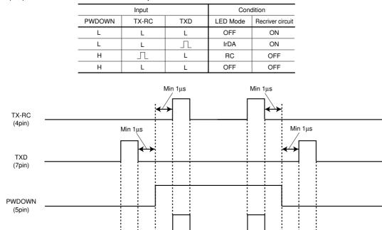
(2-b) RC transmit mode at IrDA receiver power down condition.
