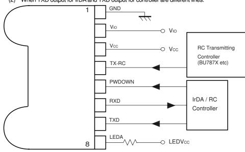
(2) When TXD output for IrDA and TXD output for controller are different lines.
