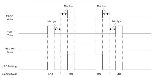
\*If TX-RC or TXD input pulse width is wider than 48µs, output LED emitting pulse will be turn off approximately 48µs.
