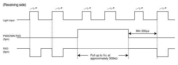
$\ast \text{RXD}$  output width is fixed approximately 2.3  $\mu\text{s}.$
