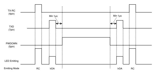
\*If TX-RC or TXD input pulse width is wider than 48µs, output LED emitting pulse will be turn off approximately 48µs.
