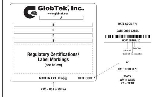
A=Medical/ITE/Household use Power Supply B=P/N: (料号) RR9KA4500T00NAIMR6B C=Model (型号) GTM96300-2307.5-2.5-R2 D=Input (输入) 100-240V~, 50-60 Hz, 1A E=Output (输出)5 V == 4.5 A,22.5W
