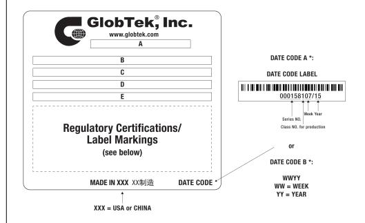
A=Medical/ITE/Household use Power Supply B=P/N: (料号) RR9KG2400T00NAIMR6B C=Model (型号) GTM96300-3619.5-4.5-R2 D=Input (输入) 100-240V~, 50-60 Hz, 1A E=Output (输出)15 V === 2.4 A ,36.0W
