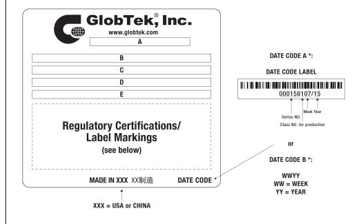
A=Medical/ITE/Household use Power Supply B=P/N: (料号) RR9KH2000T00NAIMR6B C=Model (型号) GTM96300-3624-6.0-R2 D=Input (输入) 100-240V~, 50-60 Hz, 1A E=Output (输出)18 V === 2 A ,36.0W
