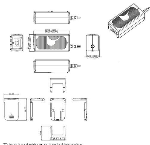
Units shipped without an installed input plug have a "desktop insert" installed.
