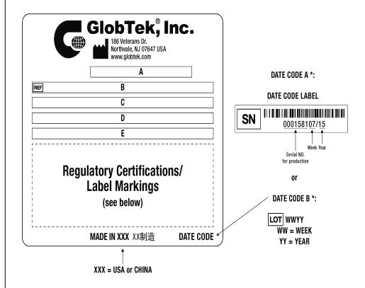
A=Medical/ITE/Household use Power Supply B=P/N: (料号) RR9LH2000T00NACIMR6B C=Model (型号) GTM96300-3619.5-1.5-R3A D=Input (输入) 100-240V~, 50-60 Hz, 1.0A E=Output (输出)18 V === 2.0 A,36.0W
