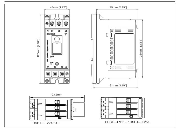
Soft Starter Three-Phase Scroll Compressor Soft Starter Types RSBT
