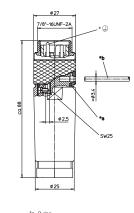
\*a O-ring \*b Pin or screwdriver as assembly tool \*⊕Contact 1.5 leading
