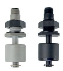
The RSF150 series are compact vertically mounted devices with a single switch point. Mounting is either from the top or bottom of a tank from the inside, so requires access to the inside of the tank.
