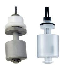
RSF50 series are compact vertically mounted devices with a single switch point. Mounting is either from the top or bottom of a tank from the inside, so requires access to the inside of the tank.
