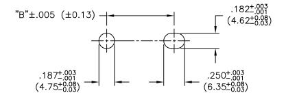
RECOMMENDED MOUNTING HOLES PANEL THICKNESS: .047-.090 (1.2-2.3)
