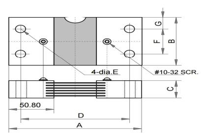
\*Dimension tolerances: ±0.381mm for hole diameters. All other dimensions have a ±0.762mm tolerance
