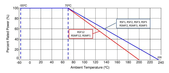
General Purpose Metal Oxide Resistor
