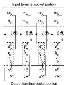
Note: The polarities of the output terminal socket are for the DC only type (equipped with AQZ102\*)
