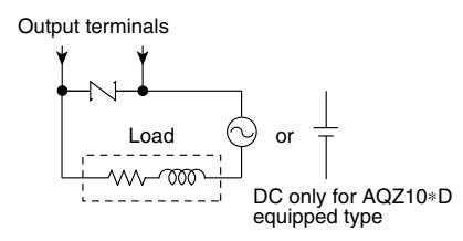
4) Even if spike voltages generated from the load are limited by a clamp diode or R-C snubber, inductances in long circuit wires will still create spike voltages. Keep wires as short as possible to minimize inductance.
