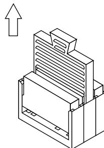
(3) Slide the removal key off of the module.
