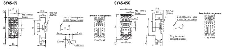
**Finger-safe DIN Rail Mount Socket**
