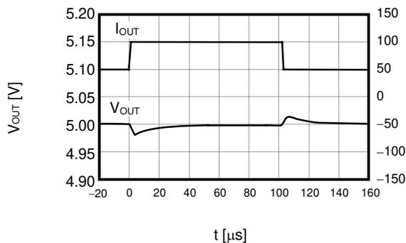
(3) Shutdown pin transient response characteristics
