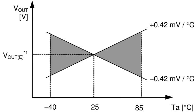
\*1.  $V_{OUT(E)}$  is the value of the output voltage measured at 25 $^{\circ}\text{C}$ .
