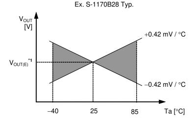
\*1.  $V_{OUT(E)}$  is the value of the output voltage measured at 25°C.
