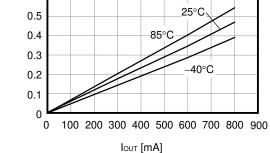
(5) Output voltage vs. Ambient temperature
