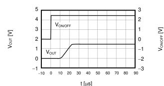
$\begin{array}{l} S{-}1170B50 \ (Ta=25^{\circ}C) \\ V{}_{IN}=6.0 \ V, \ Cout=4.7 \ \mu F, \ C{}_{IN}=4.7 \ \mu F, \ lout=300 \ mA \end{array}$
