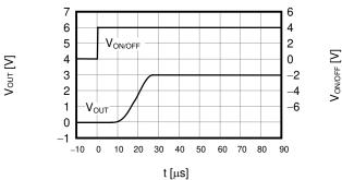
$\begin{array}{l} S{-}1170B30 \ (Ta=25^{\circ}C) \\ V{}_{IN}=4.0 \ V, \ C{}_{OUT}=4.7 \ \mu\text{F}, \ C{}_{IN}=4.7 \ \mu\text{F}, \ I{}_{OUT}=300 \ m\text{A} \end{array}$
