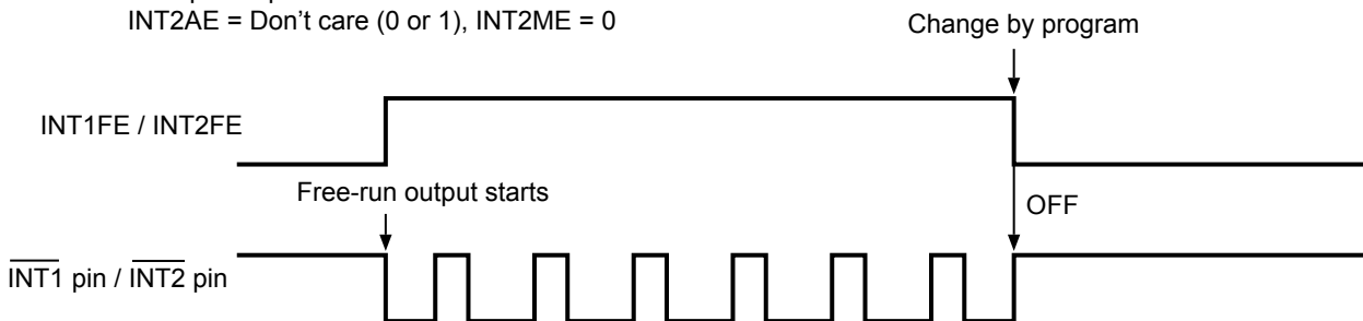
Figure 26 Output Timing of User-set Frequency
