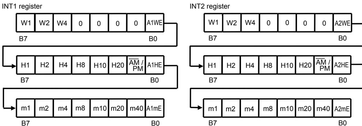
**Figure 12 INT1 Register and INT2 Register (Alarm-Time Data)**
