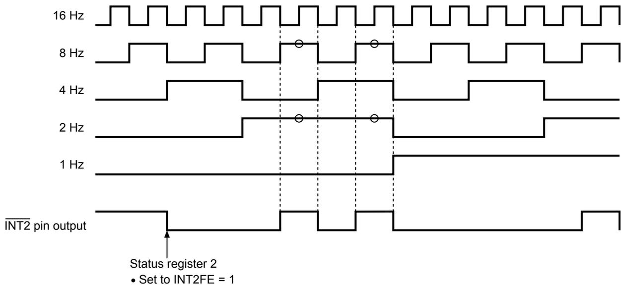
**Figure 15 Example of Output from INT2 Register (Data Register for Output Frequency)**
