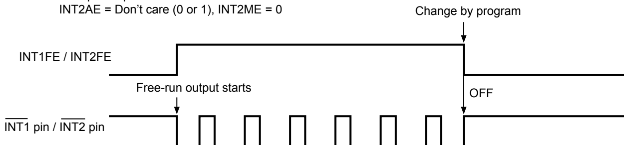
Figure 27 Output Timing of User-set Frequency
