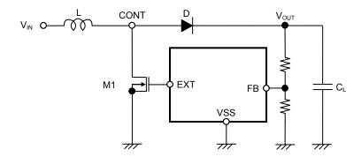
Figure 10 Step-up Switching Regulator Circuit for Basic Equations
