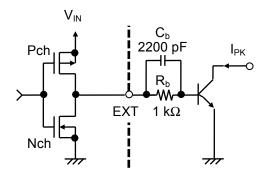
Figure 11 External Transistor Periphery
