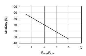
Figure 13 R<sub>Duty</sub>/R<sub>OSC</sub> vs. MaxDuty
