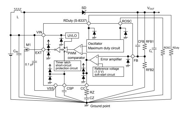
Figure 15 Standard Circuit (S-8337 Series)
