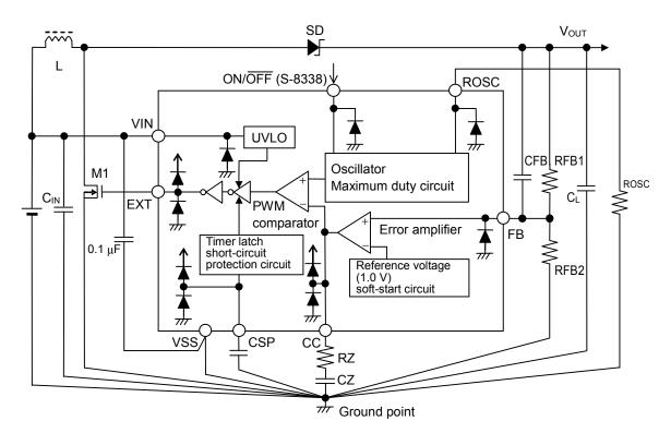
Figure 16 Standard Circuit (S-8338 Series)
